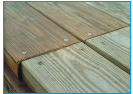
During a rainstorm, the differences between conventional treated wood (top) and Wolmanized® wood with Lumbrella™ (foreground) are obvious. The regular wood has absorbed more water, assumed a darker color, and swollen noticeably compared to the lumber with built-in water repellent.
